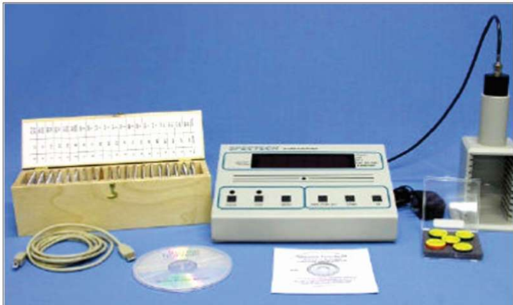
Fig. 3 Setup of a typical G-M counter.
